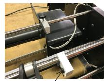
Remove screws from mounting blocks.
